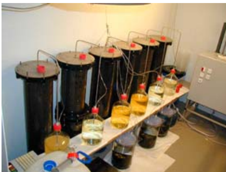
Figure 5.1. Example of up-flow percolation column test for organic compounds (photo from DHI).
